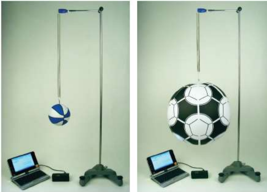
Picture 5.4.1 oscillation experiment of a spring pendulum: motions of a big ball and a small ball that have different masses and volumes
