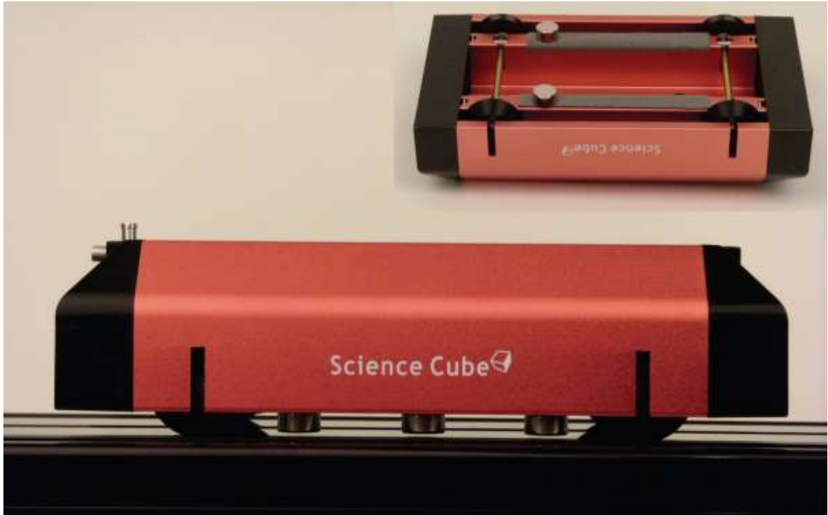
Picture 5.6.9 experiment with different damping resistances: make the damping resistance bigger by attaching magnets 109 to the cart
