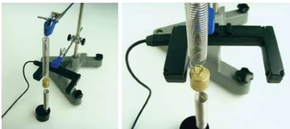
Picture 5.4.9 oscillation with two springs: Oscillate the pendulum up and down so that it blocks and unblocks the photogate.
